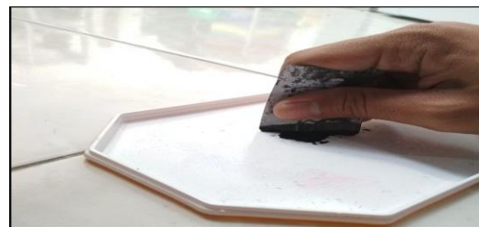
Figure 3. Mixing of conductor inks with water
