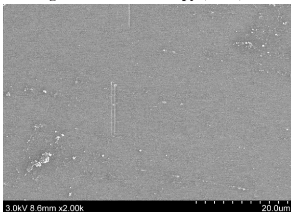
Figure 3. SEM of pure polylactide.
