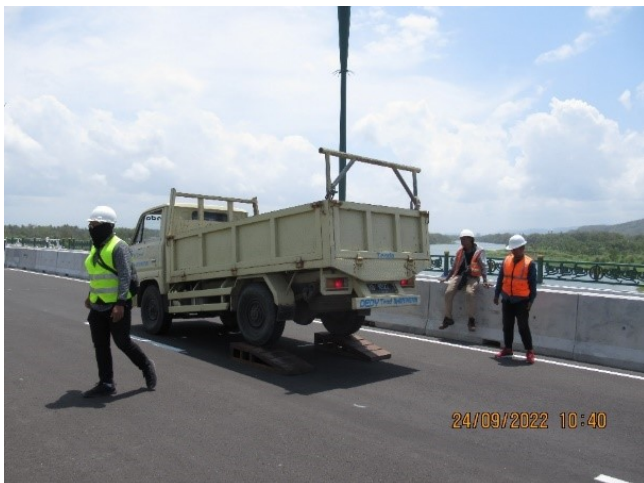
Figure 5 Impact load from truck as excitation load in dynamic load test
