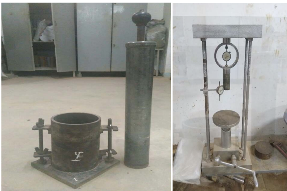
Figure 4. Standard Proctor test equipment and the CBR instrument
