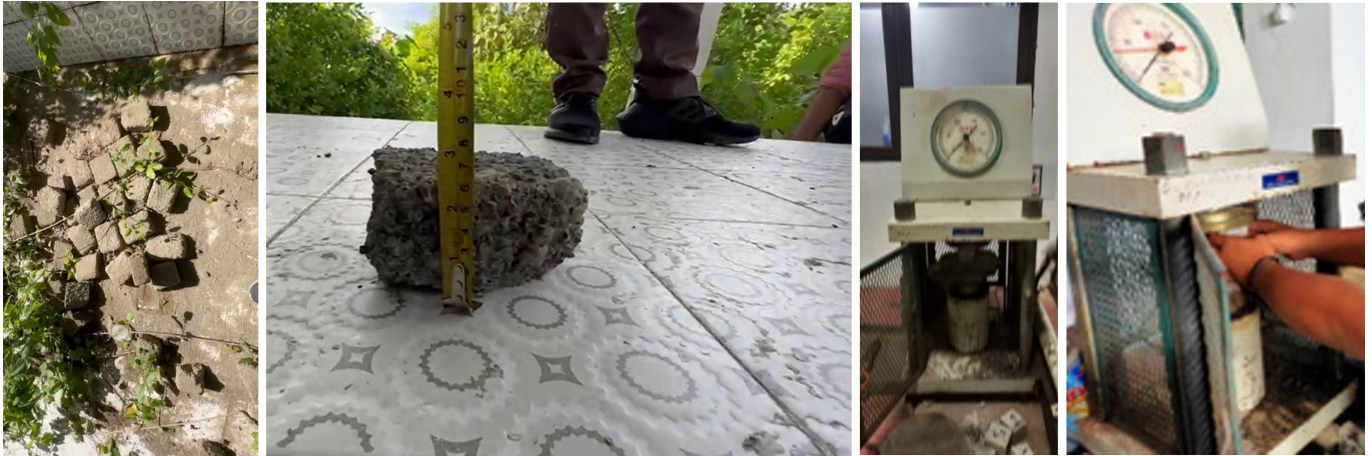
Figure 7 Compression strength testing of paving blocks sample (left) and testing apparatus (right)
