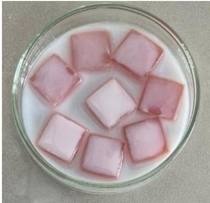
Figure 1. Coating process of acrylic resin samples with ZnO suspension in ethanol
