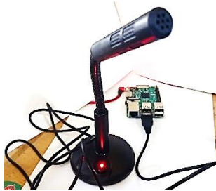
Figure 5. Raspberry Pi and microphone installation
