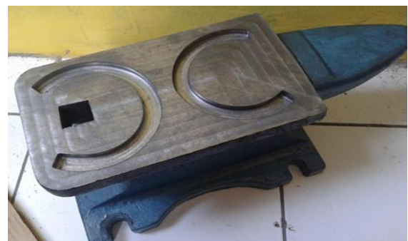
Figure 17. New tool for printing horseshoe
