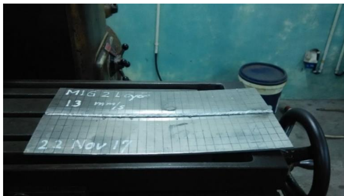
Figure 5. Welding result at welding speed of 13 mm/s
