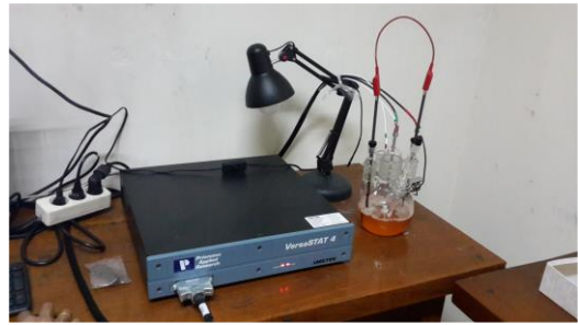
Figure 3. Potentiodynamic polarization corrosion test instrument
