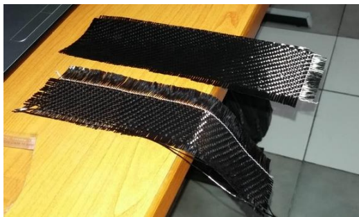
Figure 11. Difference in stiffness and thickness between pieces of woven carbon fabric
