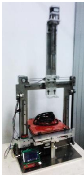
Figure 2. The aqueous based extrusion fabrication (ABEF) with RepRap controller
