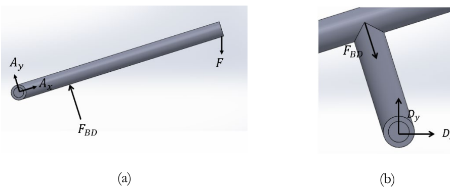
Figure 6. FBD of (a) Pipe AC and (b) Pipe BD in Top Pusher.
