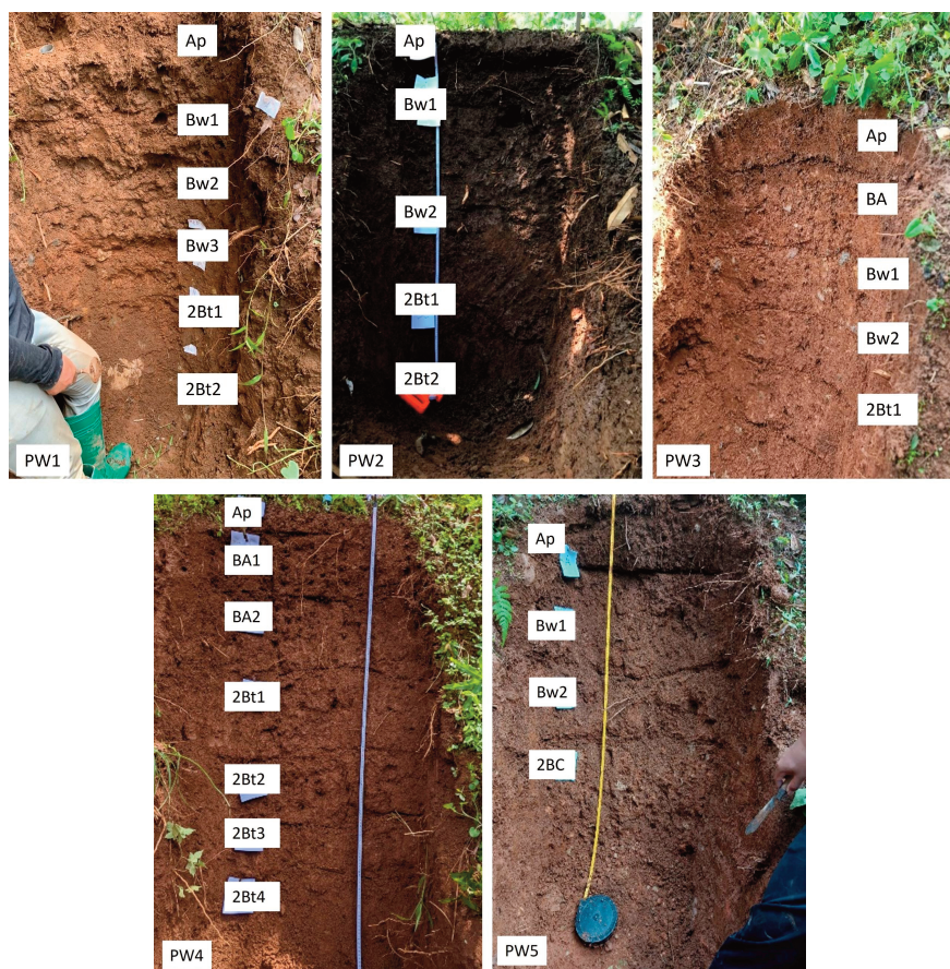
Figure 2. Soil profile in UPN experimental field (PW1, PW2, PW3, PW4, and PW5)
