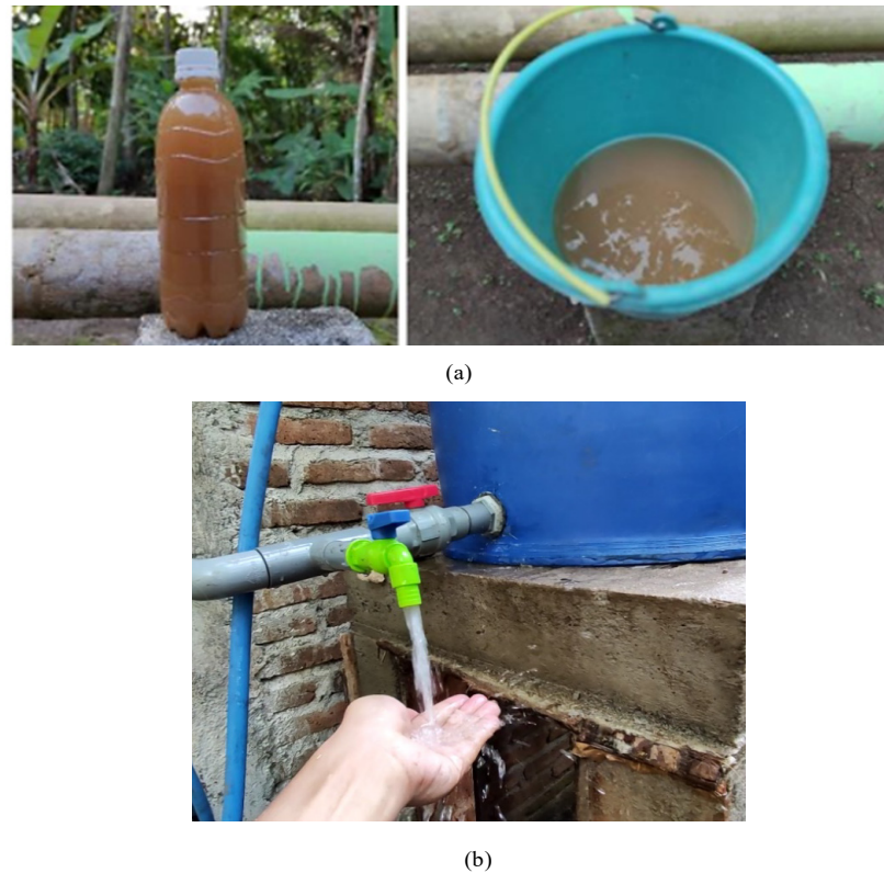
Figure 4. Comparison of water yield before and after filtration using clean water treatment technology. (4.a) The water before filtration. (4.b) The water after filtration.
