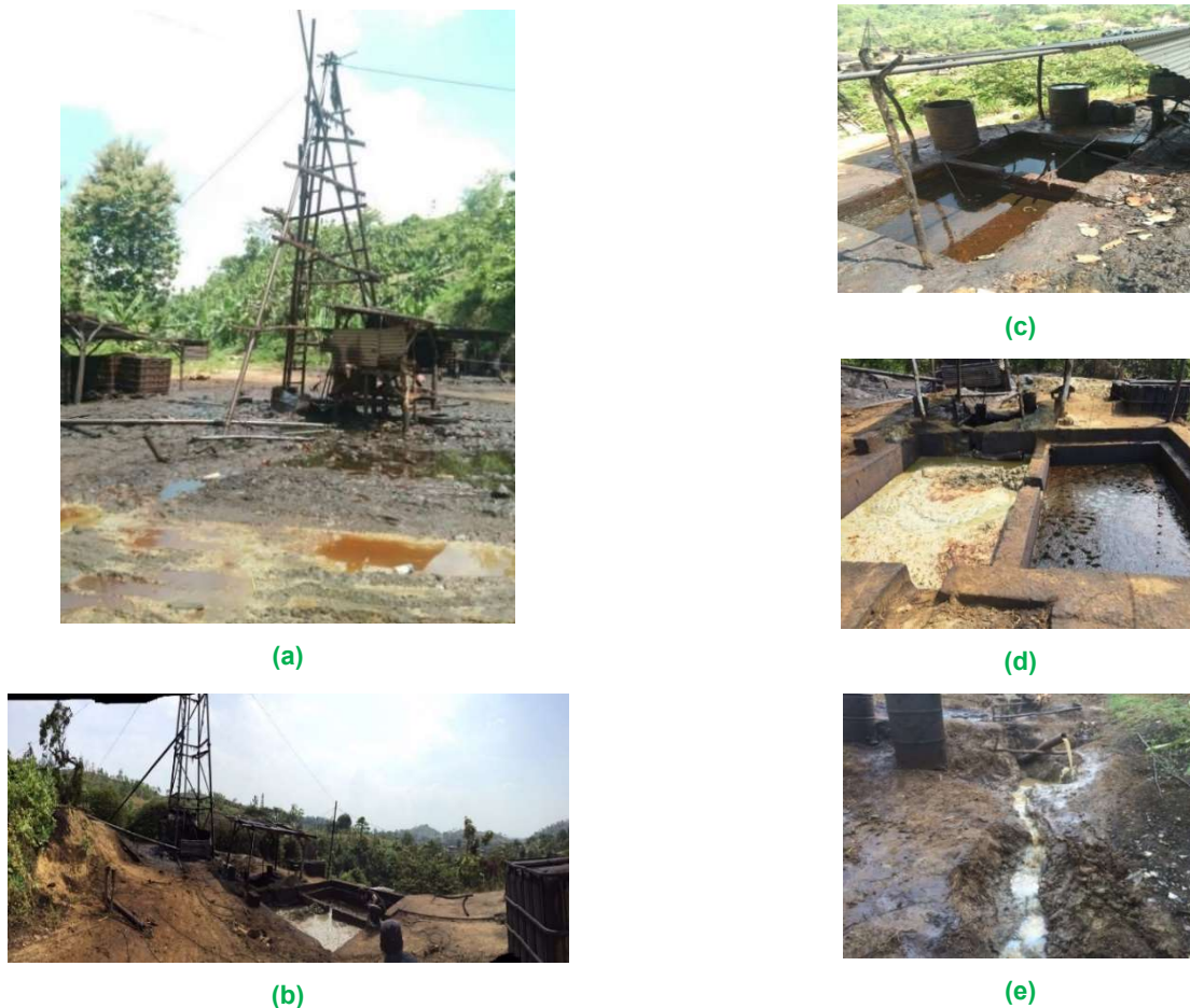
Figure 2. (a) Soil contamination in Oil Field Wonocolo, (b) Area of oil production, (c) sedimentation tank, (d) oil sludge deposition in the sedimentation tank, (e) produced water discharge to the environment after the sedimentation tank
