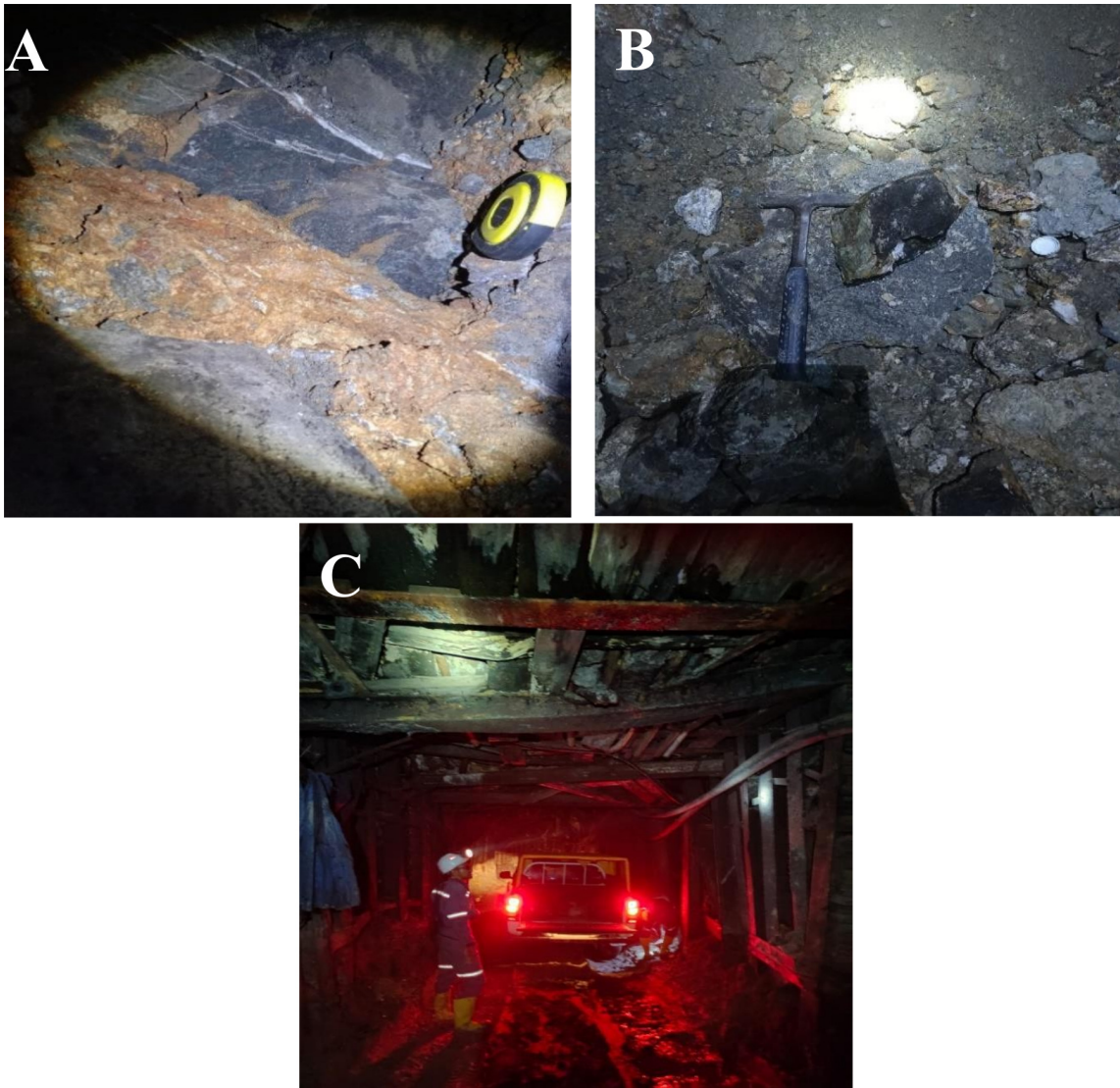
FIGURE 10. A. Long-range macroscopic appearance of contact between tuff and andesite rock units. B. Close-up appearance of Tuff and andesite rock units at XC Loop 2 and C. Actual conditions in the field at the development XC Loop 2 location.
