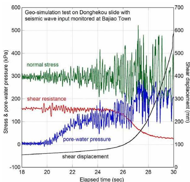
Figure 10: Zoom-up of the Geo-simulation test on the Donghekou slide.
