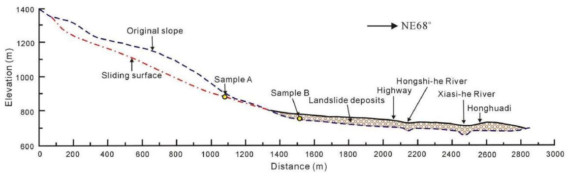
Figure 7: Longitudinal section of the Donghekou landslide
