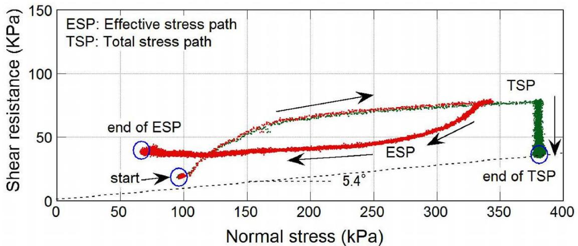
Figure 13: Total stress path and effective stress path of the simulation test with fully saturated sample B
