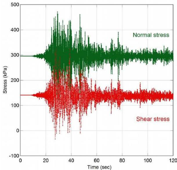
Figure 8: Real seismic wave, which was recorded by China Administration of Earthquake, was transferred to the input signal for the simulation test.
