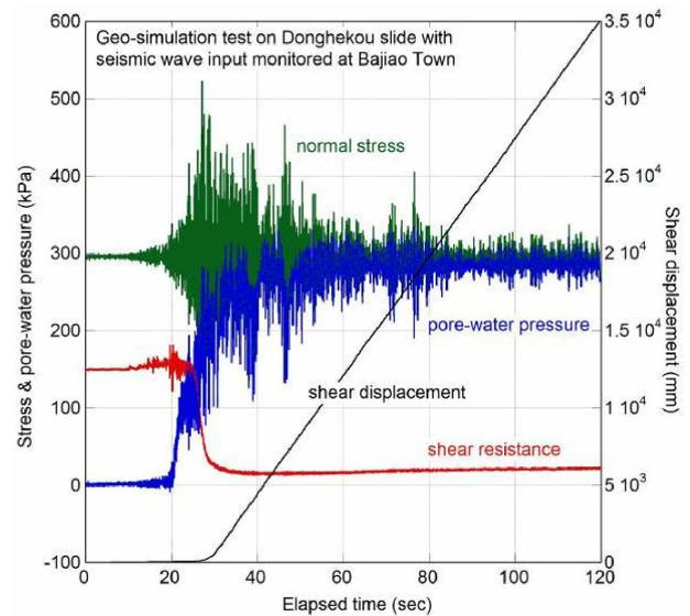
Figure 9: Geo-simulation test results of the Donghekou landslide with real seismic wave.
