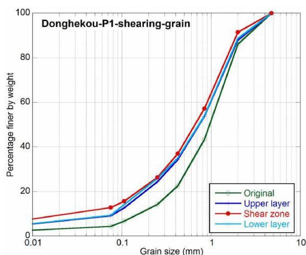
Figure 11: Grain size distribution of the source area sample from Donghekou slide. The original sample, soils from upper layer of the shear box, lower layer of the shear box, and shear zone are shown.
