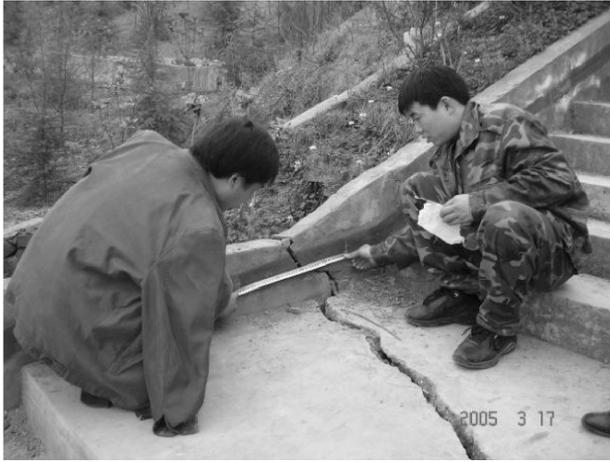
Figure 15: The ladder is cracking that is monitored and positioned by BOTDR
