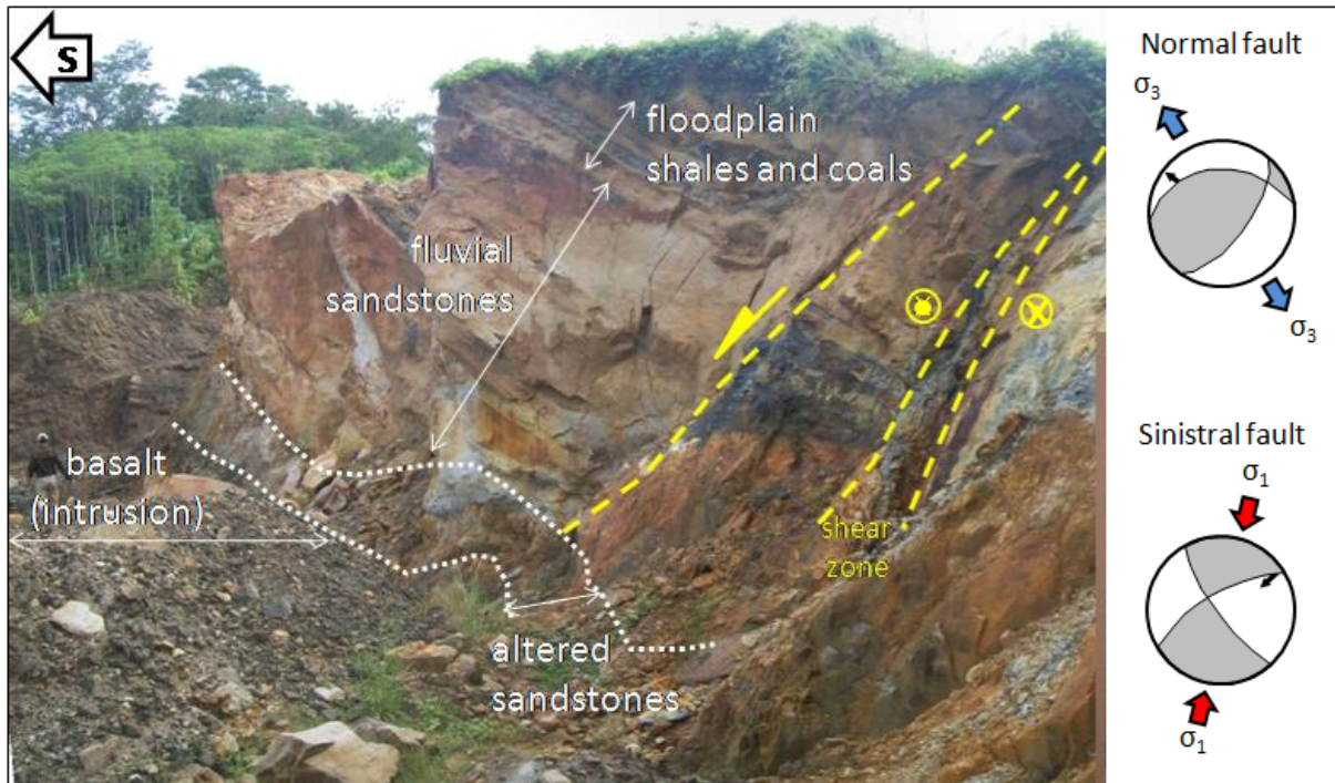
Figure 6: A 20 m thick outcrop of Tabul sandstones, intruded by basalt. Two local faults were recognized and kinematically interpreted to be related with regional tectonic framework.
