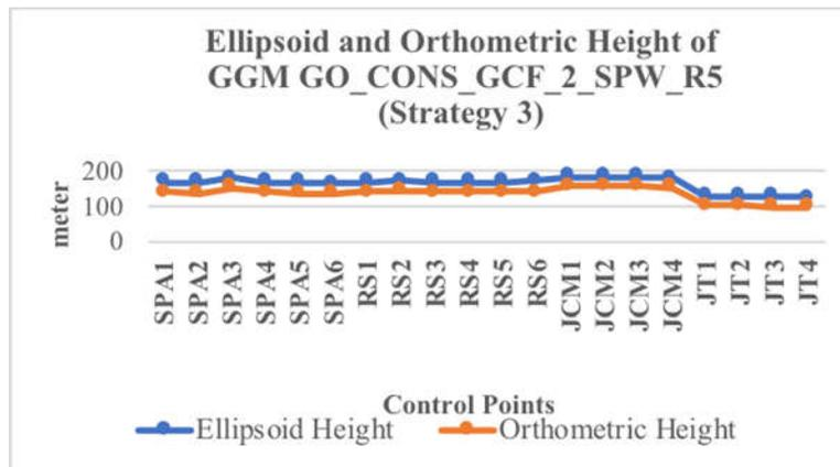
Figure 10. Comparison of ellipsoid and orthometric heights using GGM GO\_CONS\_GCF\_2\_SPW\_R5
