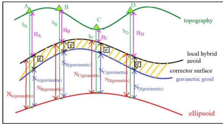
Figure 2. The process of local hybrid geoid modelling with corrector surface calculation (modified version from Nakagawa *et al.*, 2003)
