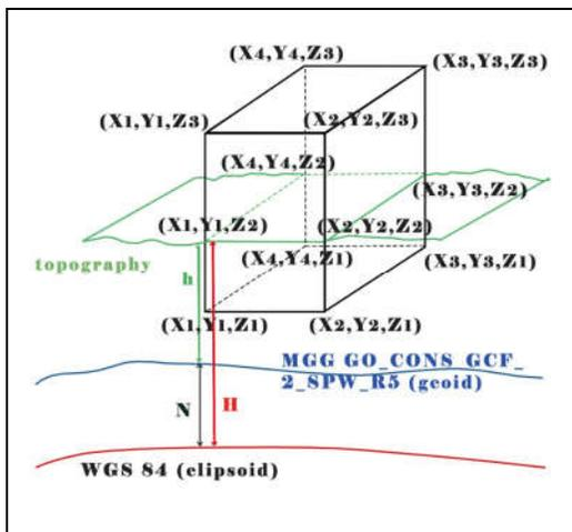
Figure 7. Geometric and orthometric heights in a 3D cadastre using GGM GO\_CONS\_GCF\_2\_SPW\_R5 hybrid geoid
