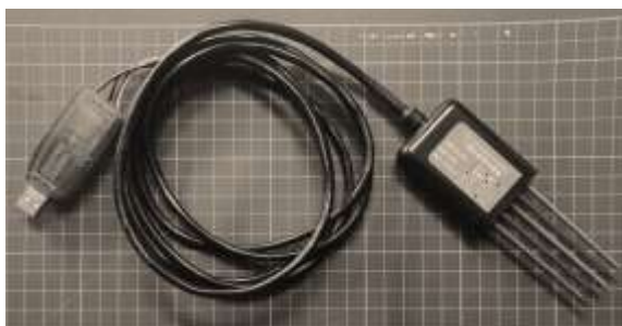
Gambar 1 Sensor NPK 普锐森社(Type 485) PR-3001-TR-ECTHPH-N01 Ver 2.0.
