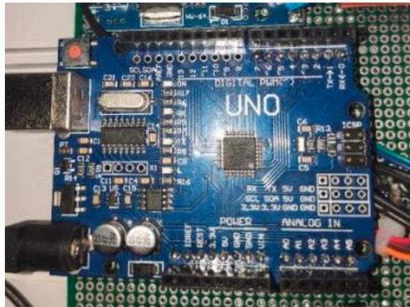
Gambar 7 Arduino Uno dan Stepdown Installation
