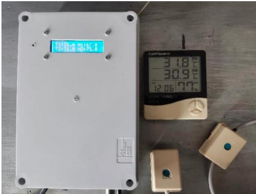
Gambar 8 DHT 11 Sensor Testing
