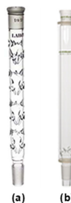
Fig 1. The (a) Vigreux and (b) Hempel columns
