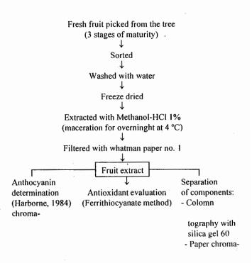
Figure 1: Fruit Preparation and Extraction
