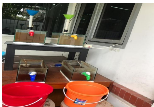
Figure 1. Anaerobic and Aerobic reactor
