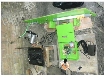
Figure 4. Actual H 2 S Monitoring System
