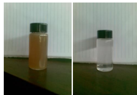
Figure 13. Effluent Before and After Screening with Membrane in COD 1800 mg/L and SRT 10 days
