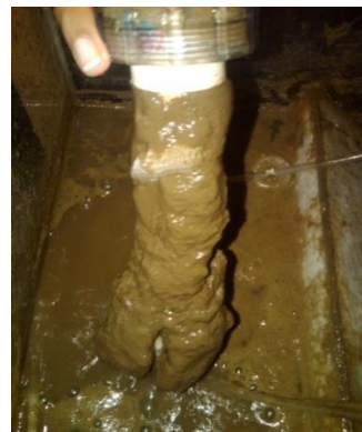
Figure 11. Fouling in SMBR
