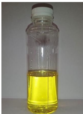
Figure 3. Appearance of FAME produced from palm oil at a temperature of 60 °C and a reaction duration of 120 minutes
