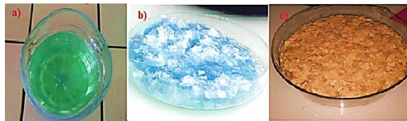
Fig. 1: (a) UP, (b) r-PET fibers, and (c) DPF fibers.
