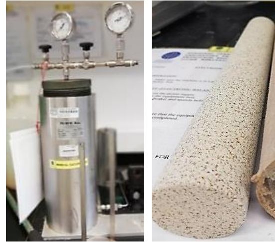
Fig. 2: Manual saturation & Buff Berea sandstone core
